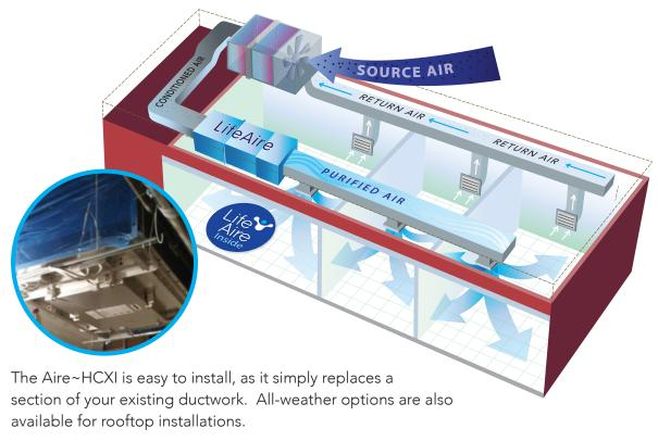
Available in three standard sizes, and able to be scaled, the Aire~HCXI efficiently services critical spaces of differing larger sizes and dimensions. All-weather options are available for rooftop installations.
